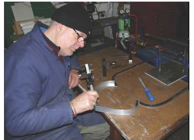
3 & 4. Stained glass frames being fabricated in the IWF Ltd workshop in Northumberland. The conservator takes a rubbing of the stained glass panel then uses this to produce a construction drawing for the fabricator. Each shaped frame takes approximately 20 hours to fabricate.
